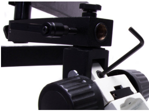
Fig. 28—Adjust the tension on the focus mount hinge using the hex key provided with the 502009 focus mount.
