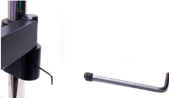
Fig. 10—(Left) The hex key is positioned inside the recessed set screw. Rotate it counterclockwise to remove the set screw.
